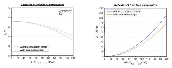
Figure 2 - Efficiency and heat loss comparative using the insulation strips proposed by KSU
