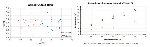
Figure 3 - Gain Output Ratio (left) and Recovery Ratio (right) vs hot inlet temperature and flow for ME-VA MD modules
