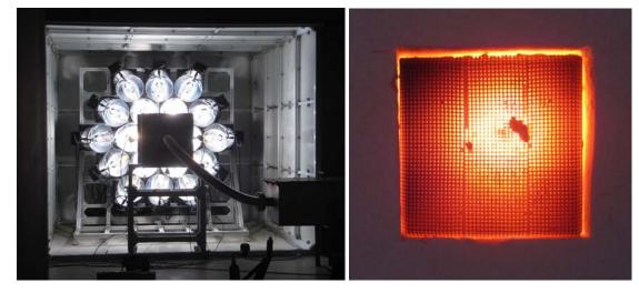
Figure 11 - Left, photograph of the IEECAS new 30 kWth high flux solar simulator during operation. Right, siliconized silicon carbide monolithic honeycomb photographed immediately after ceasing operation of the solar simulator, at temperatures in excess of 1300 °C
