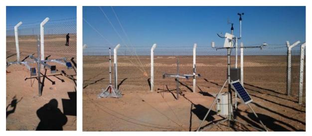
Figure 1 - Glass sand erosion holder (left) and sand particle detection device (right)
