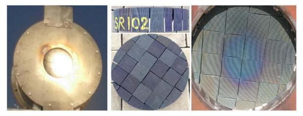
Figure 10 - Volumetric absorber material. (left) During testing; (center) before (right) after 20h
