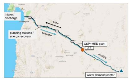
Figure 5 - Possible pipeline for inland desalination in Chile
