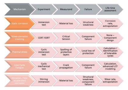
Figure 6 - Different testing routes for degradation mechanisms
