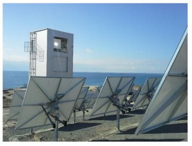
Figure 7 - CSIRO heliostats at Pentakomo facility (Cyprus)
