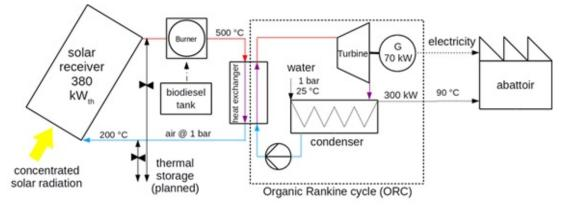
Figure 4 - Process schematic of the modified Pirassununga pilot plant
