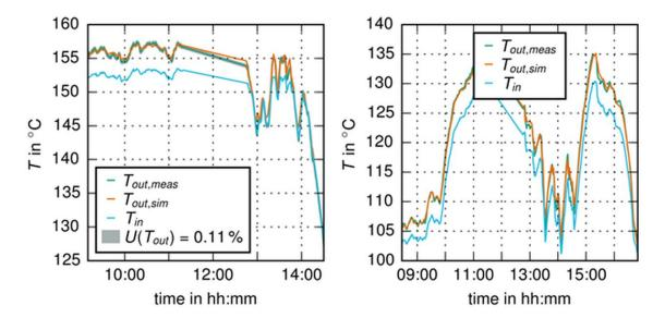
Figure 9 - Example evaluation of dynamic testing - comparison of simulation using identified parameters and measurements
