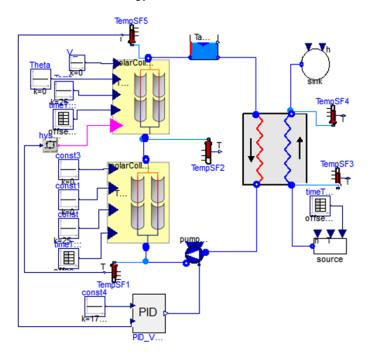
Figure 12 - Plant layout in Dymola environment simulation
